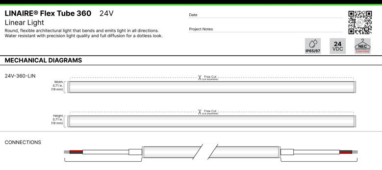
96 in. White Bare Lead 18/2 AWG UL 2464 Wire with Strain Relief
