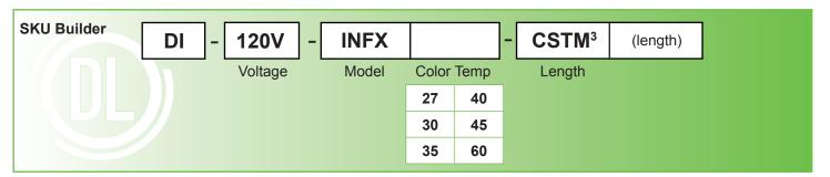
Example: DI-120V-INFX42-CSTM-20' = Diode, 120 Volt, INFINILINE®, 4,200° CCT, 20 feet custom cut.
